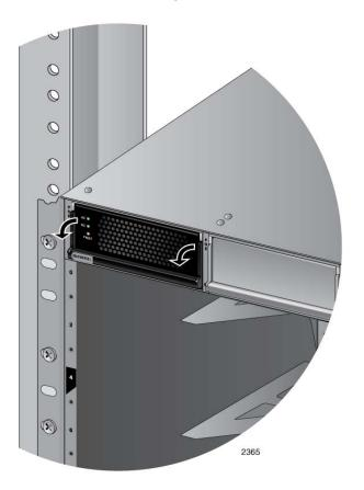
Figure 61. Locking the Handle on the AT-SBxPWRPOE1 AC Power Supply
